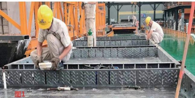
Picture 1: one-off moulding of rough surface
